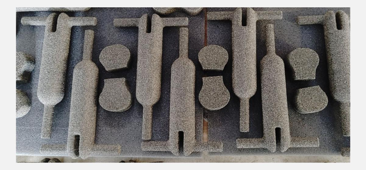
3MM THICK ADI TEST FINGER CASTING 1250MPA TENSILE, 14% ELONGATION BENT AROUND VICE FACE
