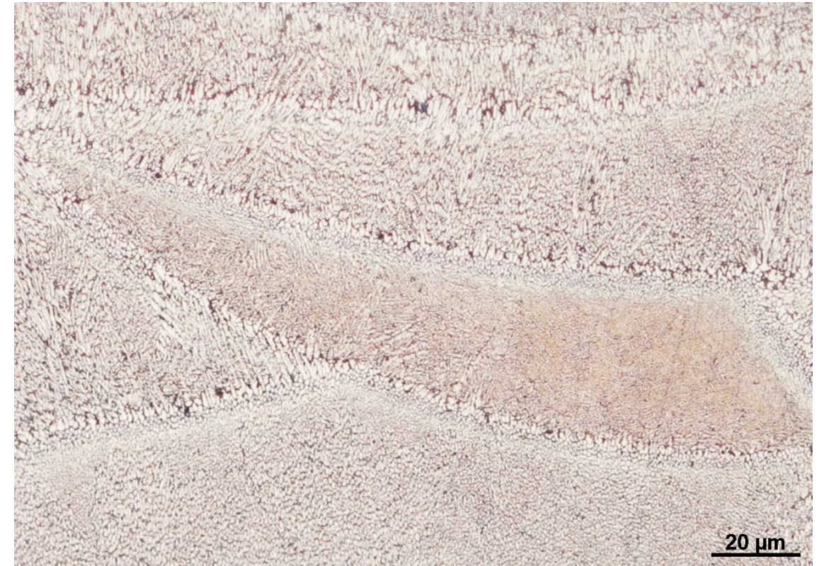
AISi10Mg, SLM, polished, Si is dispersed. Axiolmager.Z2m, BF, 500x
